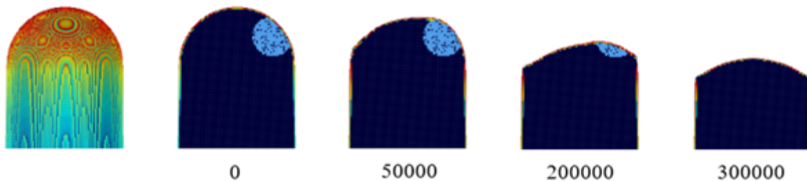
Figure 3: Evaporation sequences of a simulated Al-Fe tip with a high field precipitate.
