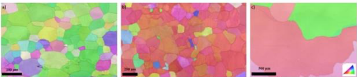
Fig. 1. Inverse pole figure, color-coded EBSD maps acquired from sample Li-1 (a), sample Li-2 (b) and Li-3 (c).
